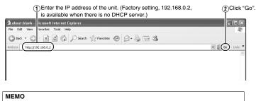
Direct specification of the IP address may not be possible when a proxy server is used for Internet access. In this case, disable the proxy setting.
