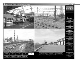
Launch Internet Explorer and enter the built-in viewer's URL in the address field again for next launch. For example, enter as follows if the IP address of VN-E4 is 192.168.0.2.
