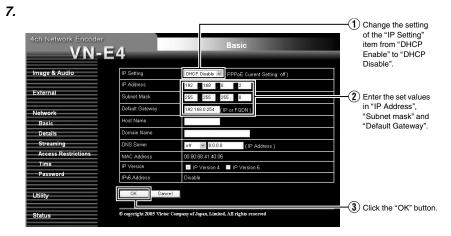
Click the "OK" button when the confirmation screen is displayed. This changes the IP address of VN-E4 to the new setting. Upon changing the IP address for VN-E4, access from this PC may fail. In order to continue access to VN-E4 from the same PC, alter the IP address of the PC accordingly.
