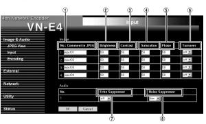
This page can be used upon access via "admin" or "operator". Press the "OK" button to enable the new settings upon changing. If the "OK" button is pressed upon entering an invalid value, a warning message will appear and entry will be denied. Press the "Cancel" button to restore the invalid entry to the current value.
