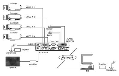
In addition to monitoring images of the 4 channels, bi-directional audio conversation is also possible. When there is alarm input and detected motion, these will be displayed on the viewer. A warning light may be connected to the alarm output terminal, which may be illuminated upon alarm input. Images that are currently displayed may be captured in the PC's hard disk.
