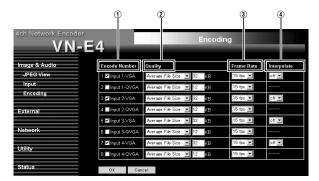
This page can be used upon access via "admin" or "operator". Press the "OK" button to enable the new settings upon changing. If the "OK" button is pressed upon entering an invalid value, a warning message will appear and entry will be denied. Press the "Cancel" button to restore the invalid entry to the current value.
